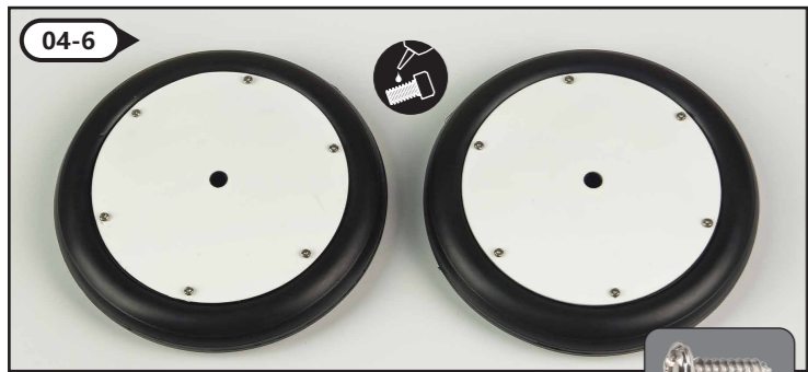
M1.6*8mm 自攻螺丝 M1.6*8mm Self-tapping screw
