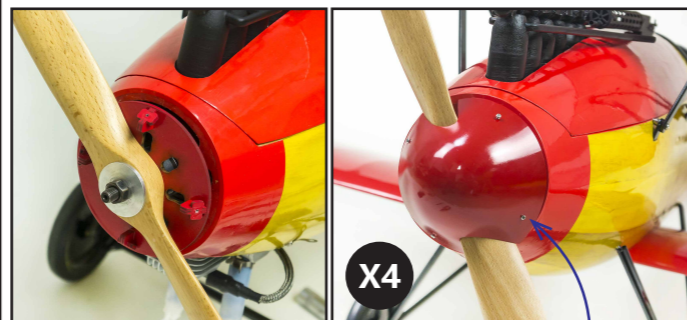
M2*10mm 自攻螺丝 M2*10mm Self-tapping screw
